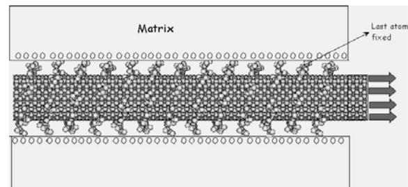
Figure 9: Schematic of the boundary conditions applied in the pullout test simulation.
