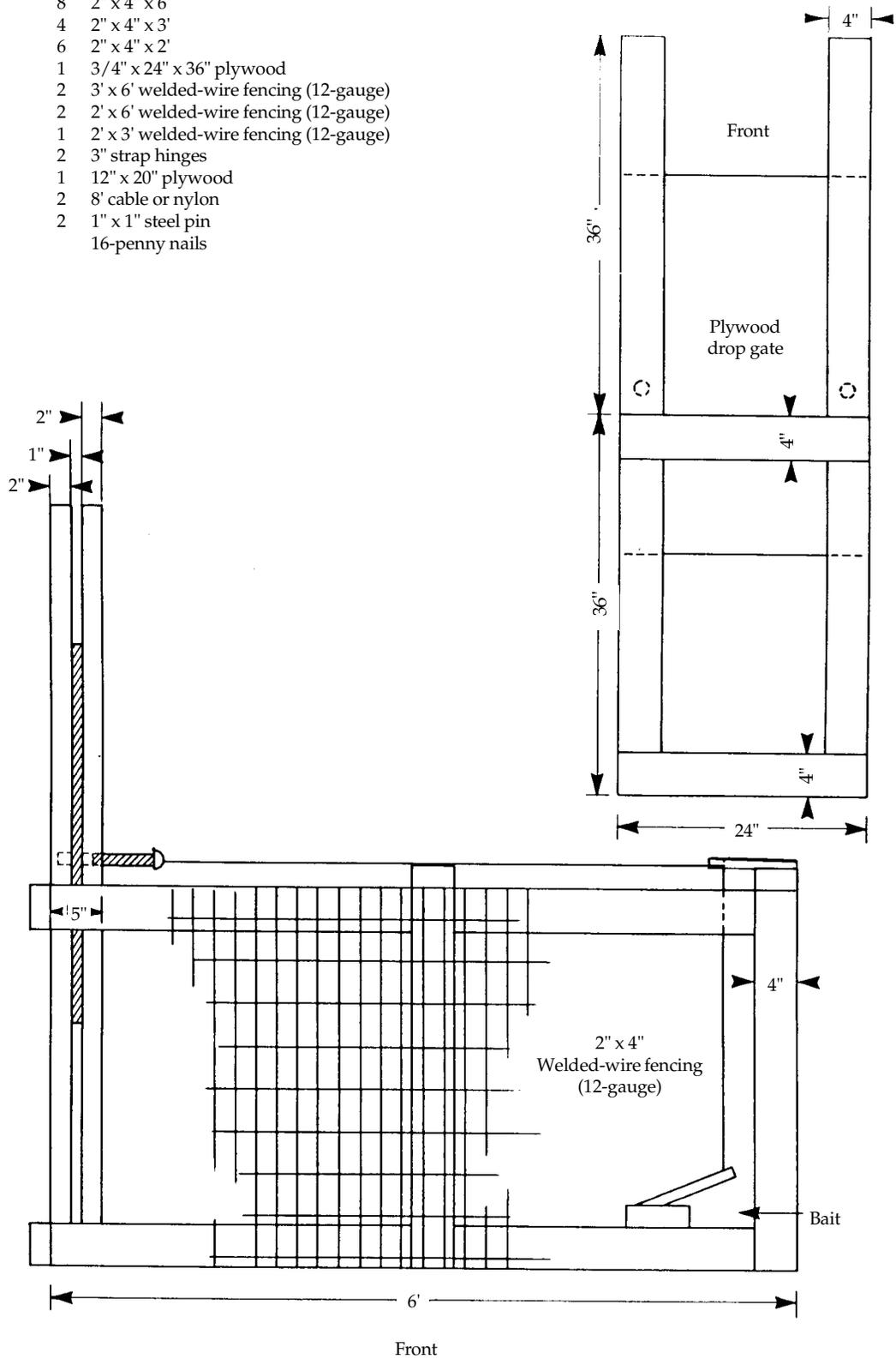
Fig. 4. Portable hog trap with drop gate
