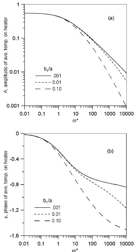
**Fig. 8** Amplitude (a) and phase (b) of the spatial average temperature on the heater as a function of frequency at  $B_a=1$  for various thicknesses of films on a large substrate. For the films,  $(\rho c)_1/(\rho c)=1$ .
