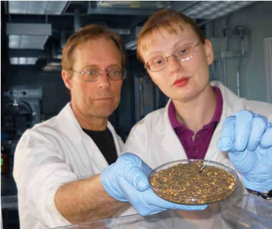
Food technologist Carl Olsen places olive pomace into a pilot-scale microwave-convection drying system while agricultural engineer Rebecca Milczarek inserts a temperature probe into it. Milczarek is studying the drying dynamics of pomace to help reduce its weight and shipping cost.
