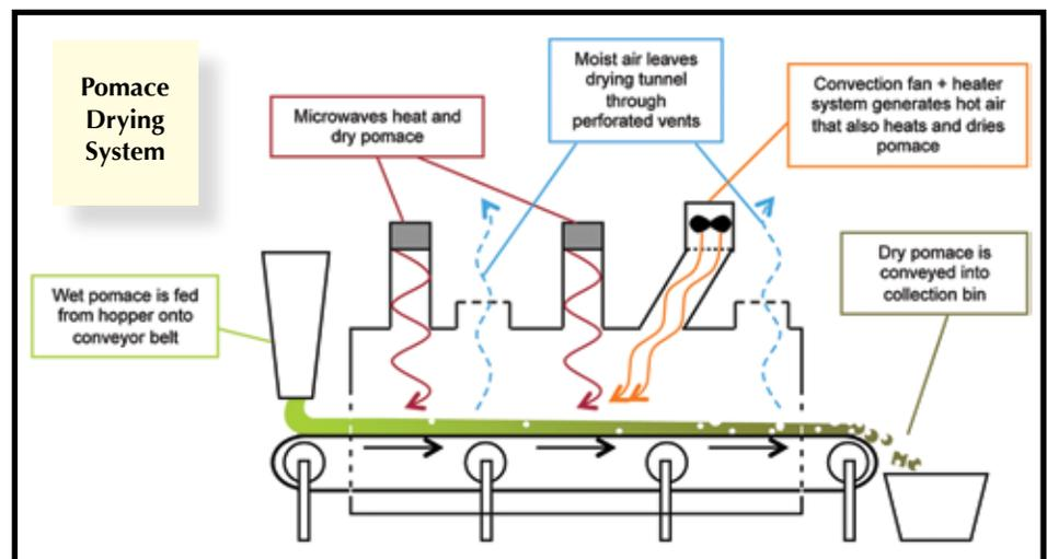
Concept diagram of an industrial continuous microwave convection drying tunnel for olive pomace. Olive processors could use findings from ARS research to define key parameters of this system, such as the speed and width of the conveyor belt.
