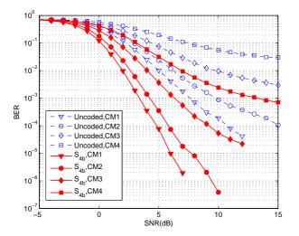
Fig. 5. QOSTFC  $S_{4b}$  with 2 Rx antennas, QPSK modulation/demodulation, and data rate 320 Mbps.
