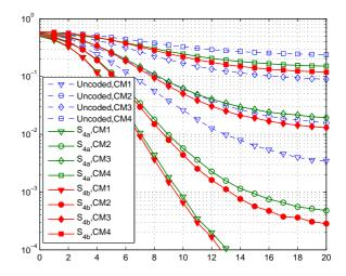
Fig. 3. STFC  $S_{4a}$  vs. QOSTFC  $S_{4b}$  with 2 Rx antennas and bit rate 480 Mbps.
