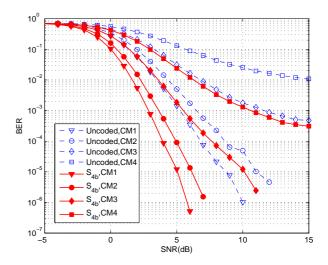
Fig. 7. QOSTFC  $S_{4b}$  with 2 Rx antennas, DCM modulation/demodulation, and data rate 320 Mbps.
