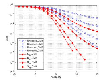
Fig. 4. QOSTFC  $S_{4b}$  with 1 Rx antenna, QPSK modulation/demodulation, and data rate 320 Mbps.
