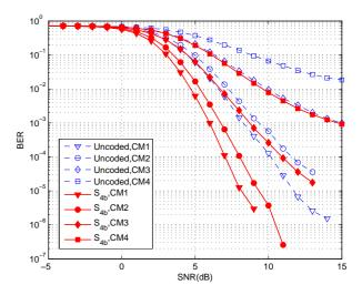
Fig. 6. QOSTFC  $S_{4b}$  with 1 Rx antenna, DCM modulation/demodulation, and data rate 320 Mbps.
