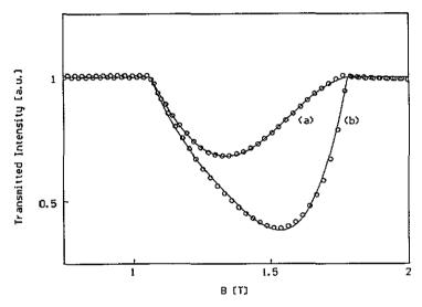
Figure 1. Transmitted intensity versus applied field (O) for + polarized light (curve (a)) and - polarized light (curve (b)) measured for FeCl<sub>2</sub> at T = 10 K and least-squares fits (——) by the use of equation (17) (a.u., arbitrary units).
