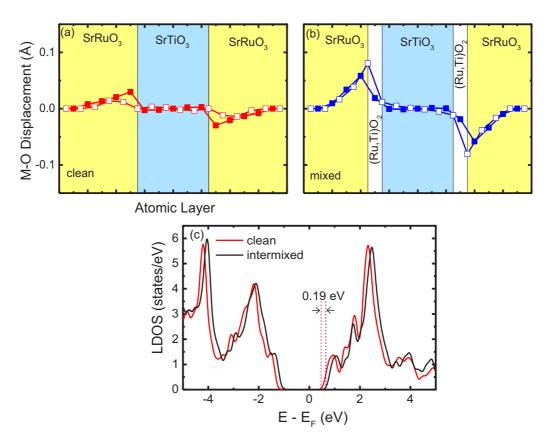
FIG. 5. Layer-by-layer metal-oxygen displacements for the two  $SrRuO_3/SrTiO_3$  supercells used to simulate the (a) T-Nb:STO and (b) S-Nb:STO interface. Solid symbols indicate the (Ru or Ti)O<sub>2</sub> displacements and the open symbols are for the SrO layers. (c) The local density of states in the center of the SrTiO<sub>3</sub> for both interface terminations. Vertical dashed lines indicate the position of the conduction-band minimum (CBM) with respect to the Fermi level,  $E_F$ .
