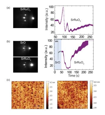
FIG. 1. Growth of 8 u.c. of  $SrRuO_3$  on  $TiO_2$  and SrO terminated substrates. (a) RHEED data for  $SrRuO_3$  growth on nonengineered substrate T-Nb:STO. (b) RHEED data for the growth of a monolayer of SrO followed by 8 u.c. of  $SrRuO_3$ . (c) AFM scan image of T-Nb:STO and S-Nb:STO.
