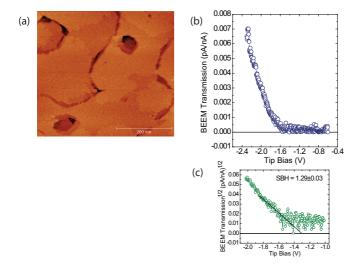
FIG. 4. (a) STM topography of 8 u.c. of SrRuO<sub>3</sub> grown on S-Nb:STO at  $V_{tip} = -1.4$  V and  $I_{tunnel} = 4$  nA. (b) Corresponding BEEM spectra through 8 u.c. of SrRuO<sub>3</sub> grown on S-Nb:STO. (c) The extracted local Schottky barrier height. Clearly, the local SBH matches with that extracted from SrRuO<sub>3</sub> grown inside the trenches of T-Nb:STO as shown in Fig. 3(b).
