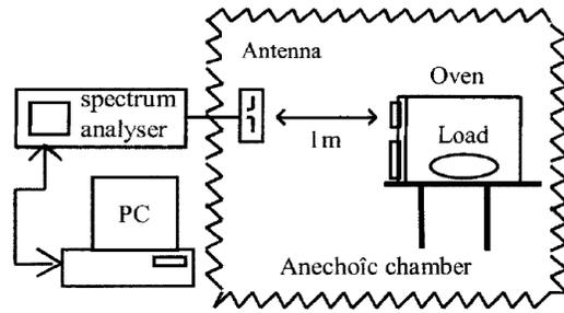
Fig. 3. Set up for magnetron frequency determination
