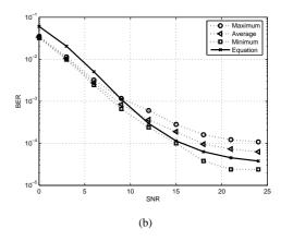
Fig. 4. MUI BER curves with Reed-Solomon coding for (a) 10 users at  $30Mbit/s,\ N_s=10$  and  $15Mbit/s,\ N_s=10$  (b) 5 users at  $30Mbit,\ N_s=5$
