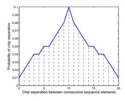
Fig. 1. ISI chip separation probabilities for Reed-Solomon codes
