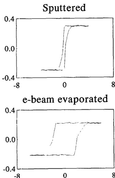
FIG. 13. The MO hysteresis loops of evaporated sample E-III-3 and sputtered sample S-I-1. The  $x$  axes are magnetic fields in kG; the  $y$  axes are Kerr rotations in degrees. The structure of the samples is  $\text{Co}(3 \text{ \AA})/\text{Pt}(10 \text{ \AA}) \times 23$ .
