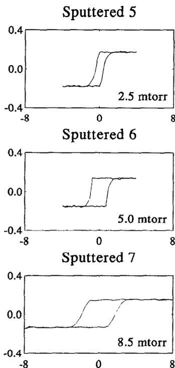
FIG. 15. Sputtering pressure effect. MO hysteresis loops of sputtered samples S-II-1, S-II-2, and S-II-3. The  $x$  axes are magnetic fields in kG; the  $y$  axes are Kerr rotations in degrees. The structure of the samples is  $\text{Co}(3 \text{ \AA})/\text{Pt}(16 \text{ \AA}) \times 16$ .
