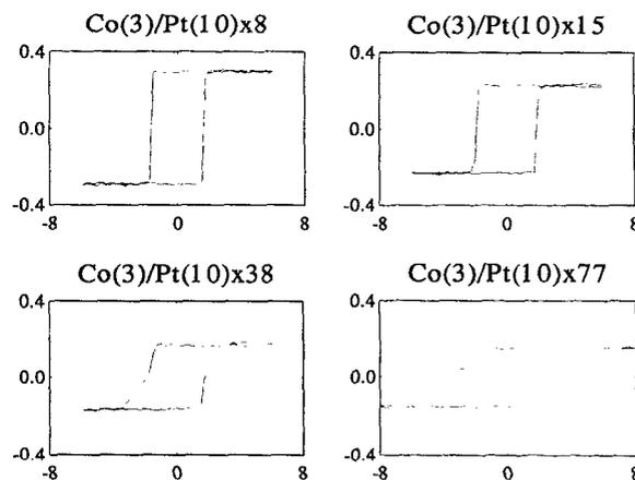
FIG. 8. MO hysteresis loops for sample group E-II. The x axes are magnetic fields in kG; the y axes are Kerr rotations in degrees.
