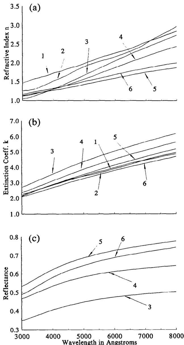
FIG. 17. (a) Index of refraction  $n$ , (b) extinction coefficient  $k$ , and (c) reflectance of samples in sample group E-II. 1: bulk Pt; 2: bulk Co; 3: sample E-II-1; 4: sample E-II-2; 5: sample E-II-3; 6: sample E-II-4. See Table I for the structures of these samples.
