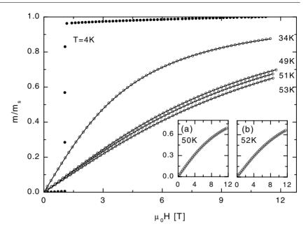
**Figure 1.** Isothermal magnetization data  $m/m_s$  versus H for FeCl<sub>2</sub> for temperatures T=4, 34, 49, 50 (inset (a)), 51, 52 (inset (b)) and 53 K. The densities of data points plotted are reduced by a factor of 50 for T=4 K and by a factor of 10 for 34 K  $\leq T \leq$  53 K. Best fits of equation (3) to the data sets for  $T \geq 34$  K are shown by solid lines.
