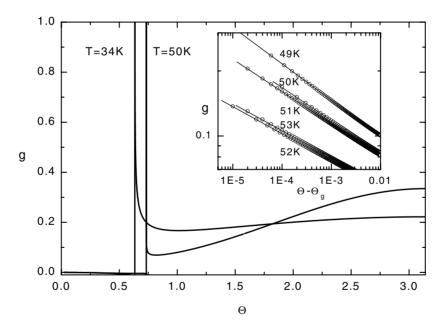
Figure 2. Selected Lee–Yang zero density functions  $g(\theta)$  for T=34 and 50 K exhibiting the temperature-dependent density gaps and the Yang–Lee edge singularities. The inset shows the density functions g versus  $\theta-\theta_g(T)$  for T=49, 50, 51, 52 and 53 K on a log–log scale. The slopes of the best-fitted power-law functions (solid lines) yield Yang–Lee edge exponents  $\mu=-0.15\pm0.02$ .
