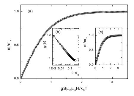
**Figure 3.** (a)  $m/m_s$  versus  $gS\mu_B\mu_0H/k_BT$  for the linear Ising chain for  $k_BT/J=100$ . The line represents the best fit of equation (1) to the data. Inset (b) shows a log-log plot of the rigorous density function [5] with the linear fit of slope  $\mu=-1/2$  in the asymptotic regime. Inset (c) shows the magnetization data (squares) with the result of the best fitting of equation (5).
