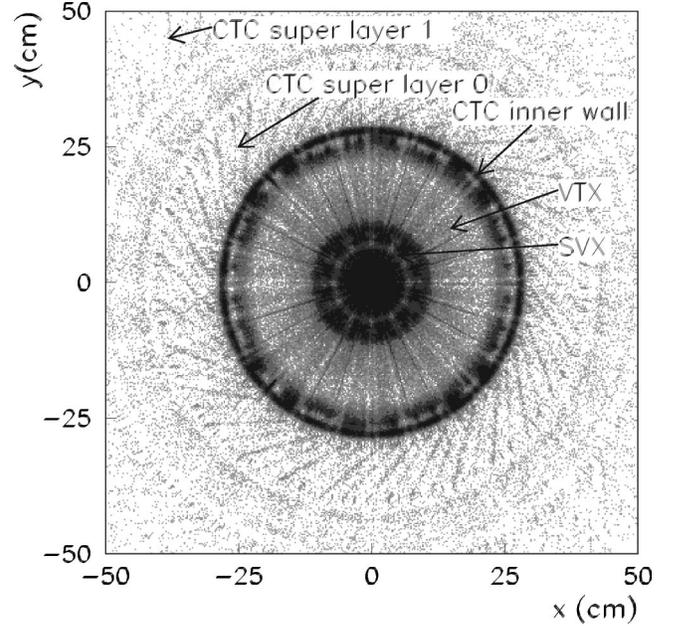
FIG. 8. Photon conversion vertex density in the  $x$ - $y$  plane in the  $74 \text{ pb}^{-1}$  of CDF run IB inclusive electron data. The fine structure of the CDF tracking detectors can be clearly resolved.
