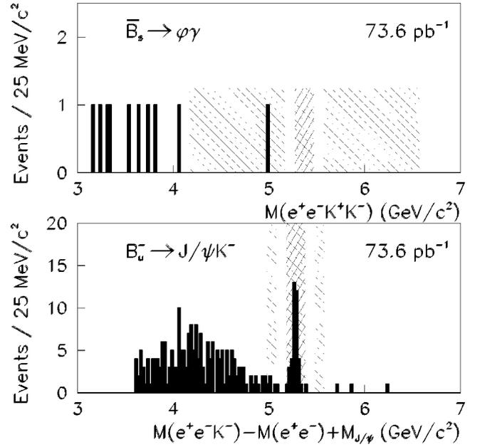
FIG. 12. Top:  $e^+e^-K^+K^-$  invariant mass distribution for  $\bar{B}_s^0 \rightarrow \phi(\rightarrow K^+K^-)\gamma(\rightarrow e^+e^-)$  in the  $74 \text{ pb}^{-1}$  of CDF run IB inclusive electron data. Bottom: corresponding  $e^+e^-K^-$  invariant mass distribution for the  $B_u^- \rightarrow J/\psi(\rightarrow e^+e^-)K^-$  reference decay. There are  $35.0 \pm 6.4$  events after background subtraction.
