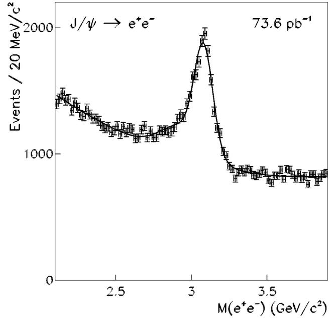
FIG. 14. Dielectron invariant mass distribution of the  $J/\psi \rightarrow e^+e^-$  candidates in the  $74 \text{ pb}^{-1}$  of CDF run IB inclusive electron data. The number of the  $J/\psi \rightarrow e^+e^-$  events obtained by fitting the mass distribution to a function of 2 Gaussians and a polynomial is  $\sim 8000$ .
