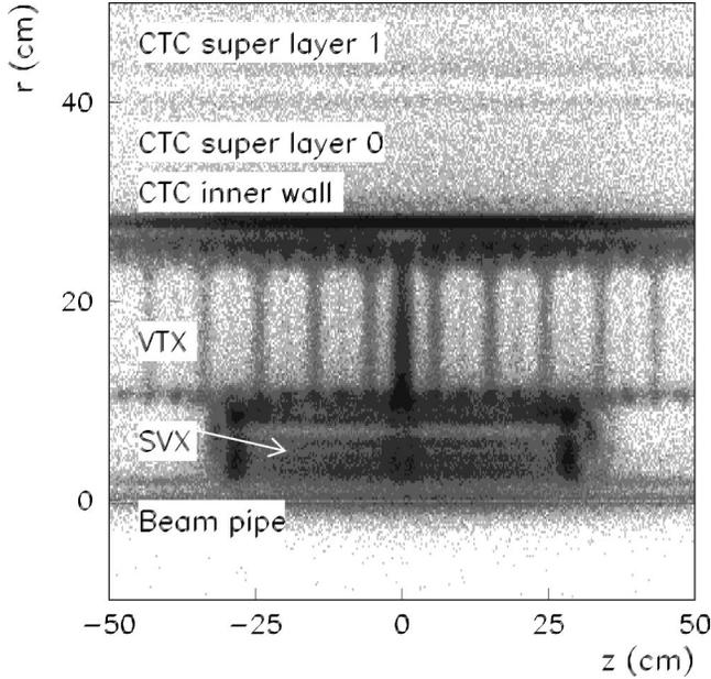
FIG. 9. Photon conversion vertex density in the  $r$ - $z$  plane in the  $74 \text{ pb}^{-1}$  of CDF run IB inclusive electron data. The fine structure of the CDF tracking detectors can be clearly resolved.
