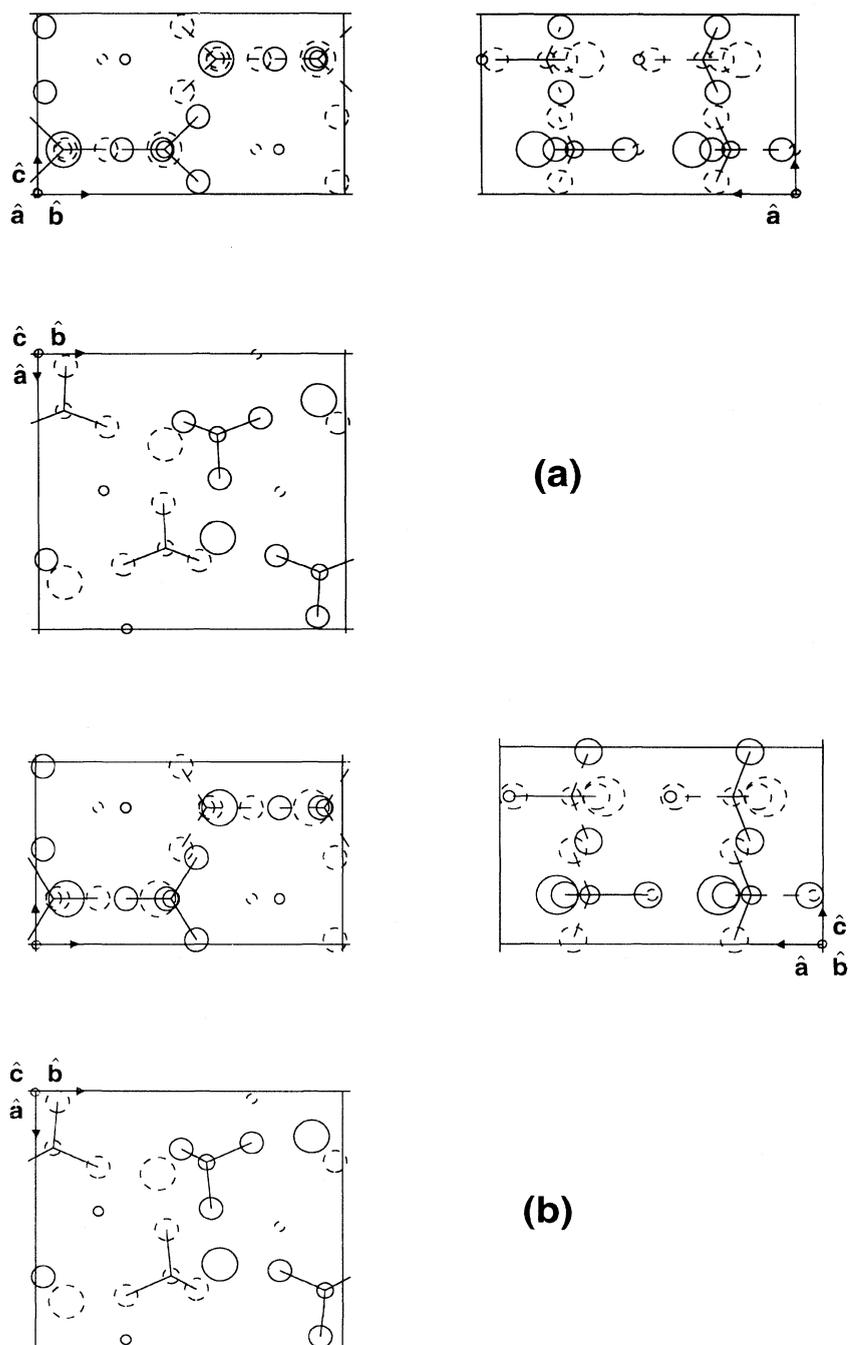
FIG. 1. Projection of the (a) experimental and (b) theoretical static structure of  $\text{RbLiSO}_4$  in the *Pnam* phase. A lattice vector pointing out of the page is represented by a circle. The smallest circles represent the Rb atoms and the largest circles represent Li atoms. Bonds (straight lines) connect each S and the nearest four O atoms. Broken lines denote ions lying above or below the plane.
