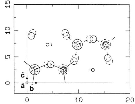
FIG. 3. Relaxed polar structure obtained by unrestricted static relaxation from the  $Pnam$  structure. Note the difference in phase between adjacent  $SO_4^{2-}$  groups compared with the  $P112_1/n$  structure in Fig. 2.
