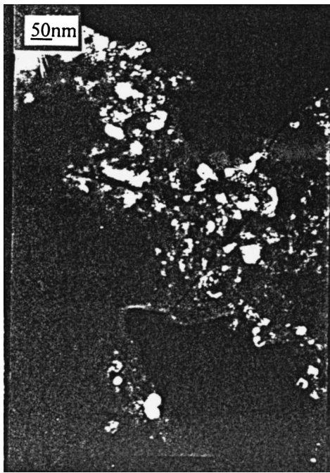
FIG. 2. Dark-field TEM micrograph of \text{Nd}_{8.4}\text{Fe}_{87.1}\text{B}_{4.5} annealed at 650^\circ\text{C} for 20 min.
