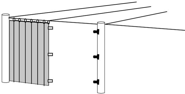
Fig. 3. Curtain-type gate for access to completely enclosed area.
