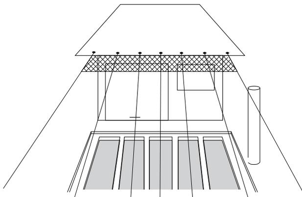
Fig. 5. Netting where wires attach to building prevents birds from walking down the roof and jumping through the wires into the facility.
