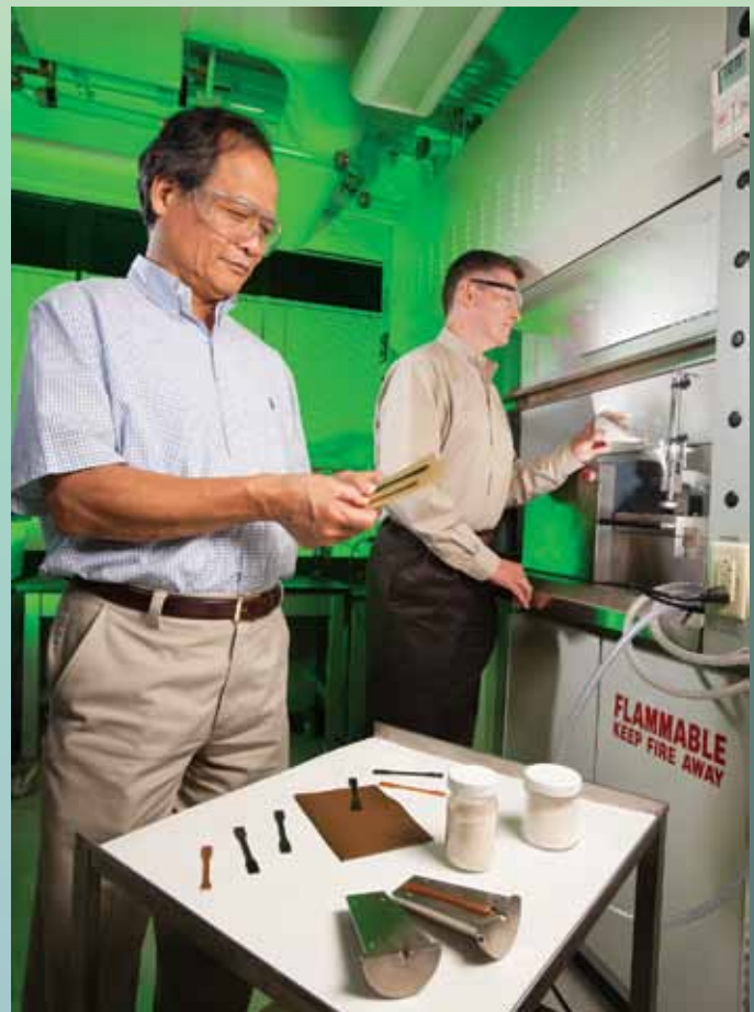
Plant physiologist Arland Hotchkiss (right) adds sugar beet pulp and poly(lactic acid) to an extruder to make the bioplastic strips that chemist LinShu Liu is inspecting.
