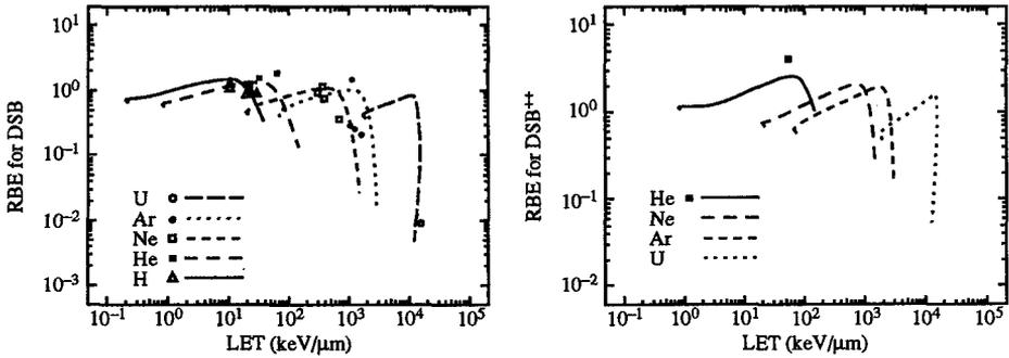
**Figure 3.** Comparison of RBE's for DSB and DSB<sup>++</sup> small deletions in radial dose model to experiments and result of the track simulation model for small deletions for He.
