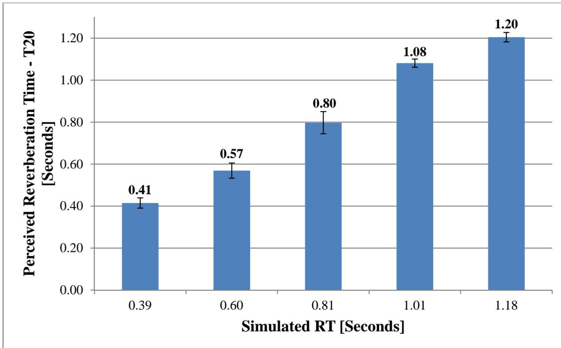
Fig. 3 – Perceived reverberation times ( $T_{20}$ ) at the listener position in the test chamber for the five reverberation time scenarios
