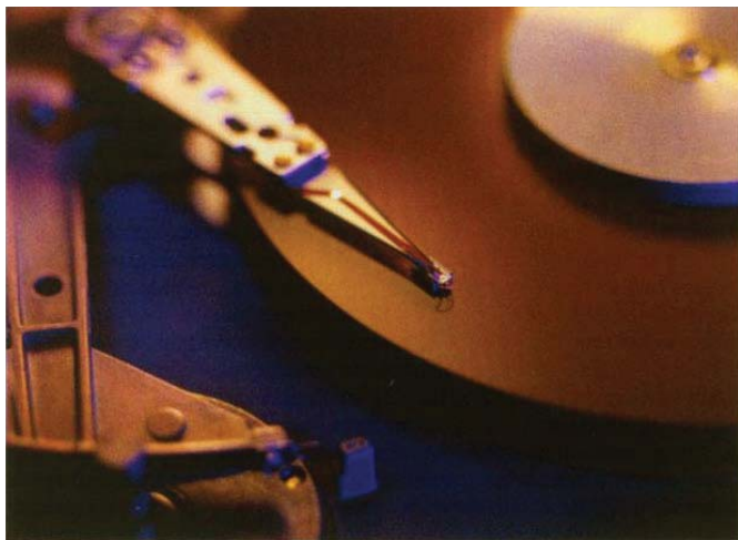
To increase the storage density of hard drives, we need smaller magnetic “bit cells” and read-heads.
