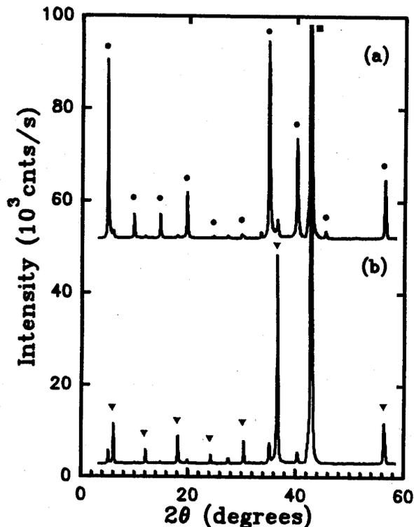
Fig. 1 X-ray diffraction patterns of Tl-Ba-Ca-Cu-O films on MgO (001) substrate. (a) annealed at 800°C (b) annealed at 790°C. (00 $\ell$ ) peaks are identified by (•) for 2223 phase and ( $\nabla$ ) for 2212 phase. (◻) for MgO.
