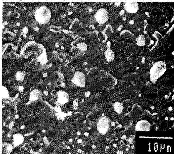
Fig. 3 SEM graph of a Tl-1223 film annealed at 810°C in vacuum.
