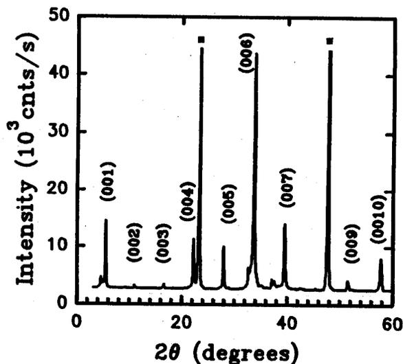
Fig. 2 X-ray diffraction pattern showing Tl-1223 phase. (00 $\ell$ ) peaks are labeled. (•) peaks are from LaAlO<sub>3</sub> substrate.
