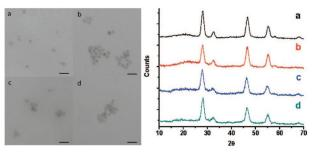
**Figure 1.** Transmission electron microscopy images (left, scale bar: 20 nm) and the X-ray diffraction patterns (right) of uncapped and capped NCs. (a) NaY $_{0.8}$ Yb $_{0.2}$ F $_4$  NCs, (b) Trop $^-$  capped NaY $_{0.8}$ Yb $_{0.2}$ F $_4$  NCs, (c) NaY $_{0.8}$ Nd $_{0.2}$ F $_4$  NCs, (d) Trop $^-$  capped NaY $_{0.8}$ Nd $_{0.2}$ F $_4$  NCs.
