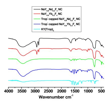
**Figure S1.** FT-IR spectra of NaY<sub>0.8</sub>Nd<sub>0.2</sub>F<sub>4</sub> NCs, NaY<sub>0.8</sub>Yb<sub>0.2</sub>F<sub>4</sub> NCs, Trop<sup>-</sup> capped NaY<sub>0.8</sub>Nd<sub>0.2</sub>F<sub>4</sub> NCs, and Trop<sup>-</sup> capped NaY<sub>0.8</sub>Yb<sub>0.2</sub>F<sub>4</sub> NCs. For comparison, the FT-IR spectra of KY(Trop)<sub>4</sub> is also depicted.
