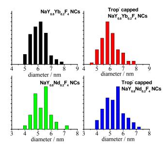
Figure S2. Histogram of the nanocrystal size distribution derived from the TEM images.
