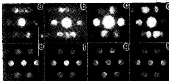
Figure 4. Comparison of TEM ( a, b, c, d ) and simulated ( e, f, g, h )  $[11\bar{2}0]$  zone axis nanodiffraction patterns. ( a ) and ( e ) : random stacking, simulation was performed using a 9-layer stacking model, ( b ) and ( f ) Two-layer stacking AB, ( c ) and ( g ) : three layer stacking ABC, ( d ) and ( h ) four layer stacking ABAC.
