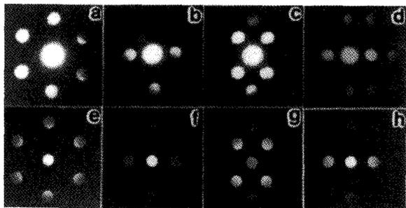
Figure 3. Comparison of TEM ( a, b, c, and d ) and simulated ( e, f, g and h ) nanodiffraction patterns. ( a ) and ( e ) :  $[0001]$  zone axis, ( b ) and ( f ) :  $[10\bar{1}1]$  zone axis, ( c ) and ( g ) :  $[20\bar{2}1]$  zone axis, ( d ) and ( h ) :  $[10\bar{1}0]$  zone axis. The simulations were performed using a three layer model ABC stacking for ( e ), and four layer stacking ABAC for ( f ), ( g ) and ( h ).
