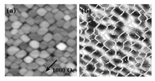
Fig. 3.  $2 \times 2 \mu m$  AFM (a) and MFM (b) images of Fe films. Images were taken under a 1000 Oe external magnetic field with a direction parallel to Ag[011] as indicated by the arrow in (a).
