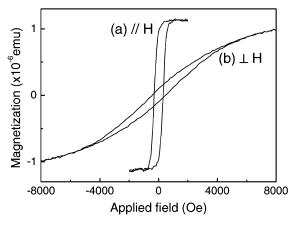
Fig. 2. Hysteresis loops of 30 nm thick Fe films grown on 40 nm thick Ag pyramidal islands. (a) and (b) are for the external magnetic field parallel and perpendicular to film plane, respectively.
