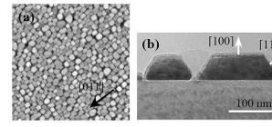
Fig. 1. (a)  $5 \times 5 \mu$ m AFM scan and (b) TEM picture of Ag pyramidal islands.
