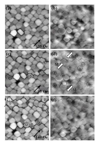
Fig. 4. A series of the  $2 \times 2 \mu m$  AFM (a), (c), and (e) and MFM (b), (d), and (f) images of Fe films under different external magnetic fields. Images (a)–(b), (c)–(d), and (e)–(f), were taken under 35, 95, and 140 Oe external magnetic fields, respectively, with a direction parallel to Ag[0-1-1] as indicated by the black arrows in (a), (c), and (e).
