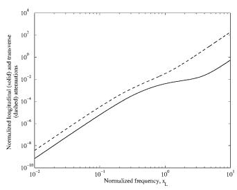
FIG. 11. Normalized longitudinal  $\alpha_L$  and transverse  $\alpha_T$  attenuations in terms of normalized frequency  $x_L$ .
