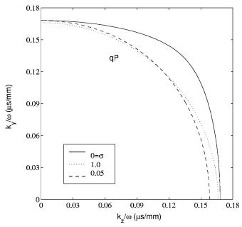
FIG. 6. Slowness surface of the quasilongitudinal wave (qP).
