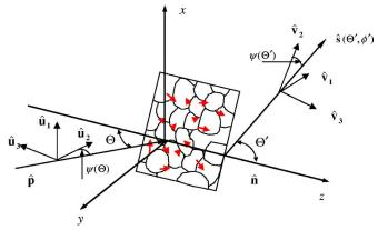
FIG. 10. (Color online) Geometry for the propagation direction  $\hat{\mathbf{p}}$ , the scattered direction  $\hat{\mathbf{s}}$ , and the respective polarization directions  $\hat{\mathbf{u}}$  and  $\hat{\mathbf{v}}$ .
