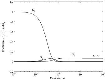
FIG. 3. Coefficients  $S_1$ ,  $S_2$ , and  $S_3$  as a function of texture parameter  $\sigma$ .
