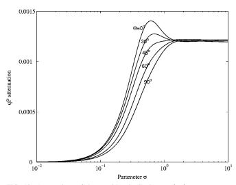
FIG. 13. Attenuations of the quasi-longitudinal wave (qP) versus texture parameter  $\sigma$  with various wave propagation directions  $\Theta$  and the given frequency  $x_{SH} = 0.5$ .
