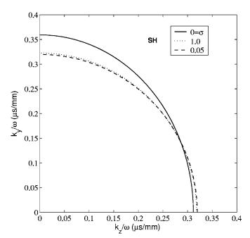
FIG. 5. Slowness surface of the shear horizontal wave (SH).
