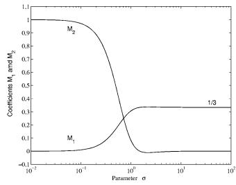
FIG. 2. Coefficients  $M_1$  and  $M_2$  as a function of texture parameter  $\sigma$ .
