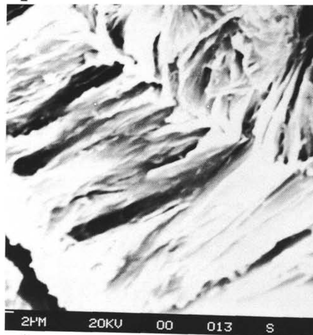
Plate 2. Laths of fibrous clay in DSDP Hole 418A basalts. 1. Sample 418A-34-3, 51-53 cm. SEM photomicrograph of X-ray diffraction mount. Laths correspond to radiating fibers seen in thin section (Pl. 1, Fig. 3) and are saponite. "Hub" of laths may be iddingsite. 2. Sample 418A-34-3, 51-53 cm. SEM photomicrograph of X-ray diffraction mount. At top center and top left, laths of saponite grade into fine-grained, platy clay. 3. Sample 418A-45-2, 40-44 cm. Standardless spectral analysis of laths seen in Figure 4. Cursor is placed approximately where K peak should be. 4. Sample 418A-45-2, 40-44 cm. SEM photomicrograph of fracture mount. Low K laths of saponite with similar morphology to those in Figures 1 and 2.
