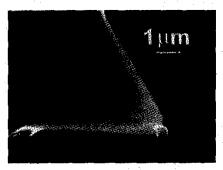
Fig. 1 A MFM cantilever with a magnet size of 500nm on the tip.
