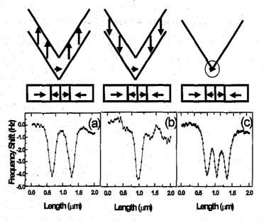
Fig. 3 Frequency shifts on 2 µm line traces across a tri-bit pattern on the reference sample with the thin-film tip (3a and 3b) and the point tip (3c). The scale of the frequency shift at Fig. 3c is 5 times less than that of Fig. 3a and 3b. The inset is the schematic drawing of the tip magnetization. The actual magnetization direction of the tip is not known. Due to the shape anisotropy of the film at tip, It is expected that have a component other than z-direction.
