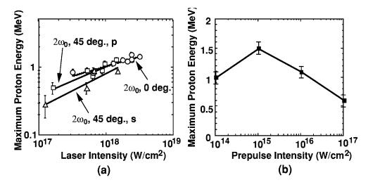
Figure 2. The maximum proton energy in the forward direction as a function of (a) laser intensity at  $2\omega_0$  and for different conditions of illumination of 1.8- $\mu$ m Al foil: circles — 0°; squares—45°, p —polarization; triangles —45°, s —polarization. Solid lines are the best power function fits to the experimental data. (b) The  $2\omega_0$  prepulse intensity at  $10^{18}$  W/cm2 main pulse intensity.
