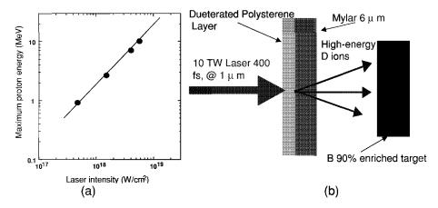
**Figure. 4.** (a) The maximum proton energy in the forward direction as a function of laser intensity  $\omega_0$ , 45°, p-polarization; (b) Schema for  $^{10}B$  activation with high-energy deuterons in the reaction  $^{10}B(d,n)^{11}C$
