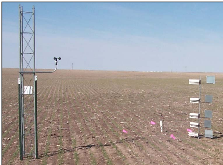
Figure 2. Station 11 was one of four stations (10-13) instrumented with BSNE samplers, a Sensit and an anemometer.
