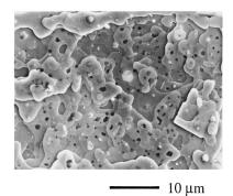
FIG. 2. Platelike grains are observed in the SEM micrograph of the (Hg,Tl)-Ba-Ca-Cu-O film annealed at 830 °C for 1 h.
