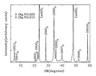
FIG. 1. The x-ray diffraction pattern for the (Hg,TI)-Ba-Ca-Cu-O film annealed at 830 °C for 1 h. The indexed peaks are for the (Hg,TI)-1223 phase and (Hg,TI)-1212 phase.
