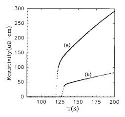
FIG. 3. Resistivity vs temperature for the (Hg,Tl)-Ba-Ca-Cu-O film (a) before and (b) after annealing in oxygen at 300 °C for 1 h.
