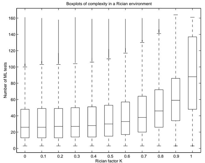
Fig. 8. Boxplots for the complexity of Asterism decoding for various values of the Rician factor  $K$ .
