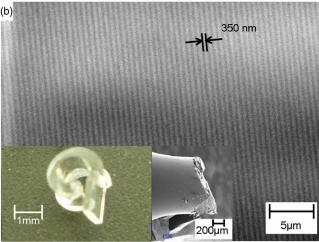
Fig. 2. SEM images of grating line features fabricated atop curved surface of portions of rigid cylinders. Insets: free-standing bilayer portions of tubes (left) and rigid replica (right). The free-standing tubular structures were received by applying uniaxial strain at 40% [(a) inset] and 80% [(b) inset], respectively.
