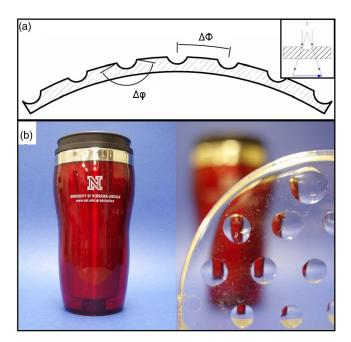
Fig. 6. (a) Illustration of a multilens imaging system with concave lenses.  $\Delta \varphi$  and  $\Delta \Phi$  are parameters related to the increment of FOV and (b) reduced images produced by an array of lens, each one focused on different locations of the object.
