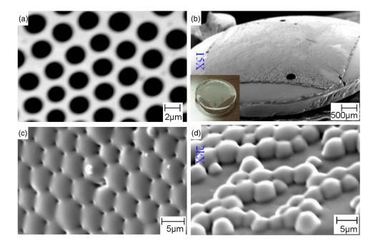
Fig. 5. SEM images of (a) polystyrene mold with close-packed features; (b) the portion of sphere structure with microlens array; (c) top view of the zoom-in image at the center of the portion of sphere, where the close-packed arrays can be seen; and (d) sideview along the edge of the portion of sphere, where a loosely packed location was picked to show the profile of individual structures for microlenses.
