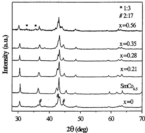
FIG. 1. X-ray diffraction patterns for  $\text{SmCo}_{7-x}\text{Ti}_x$  compounds.
