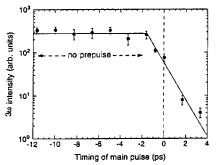
Fig. 6: Relative efficiency of 3w from flat Si vs. prepulse/main pulse delay. Prepulse is 5% of the main pulse, which is  $5 \times 10^{17}$  W cm<sup>-2</sup>.
