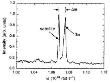
Fig. 8: The appearance of the first red-shifted satellite to  $3\omega$  from a parylene-N target (CH);  $I = 4 \times 10^{17}$  W cm<sup>-2</sup>,  $\Delta \omega = 7.4 \times 10^{13}$  rad s<sup>-1</sup>.
