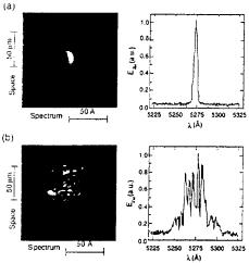
Fig. 3: Spatially resolved  $2\omega$  spectrum: (a) with clean pulse; (b) with  $10^{-1}$  prepulse. At left is a spectrum (resolved horizontally) for a slit-image of the plasma (vertically), from center of the laser focus; at right is a lineout of the spectrum through centre.
