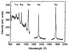
Fig. 4: Typical time-integrated harmonic spectrum from Si target, I ~  $3.2 \times 10^{17}$  W cm<sup>-2</sup>.
