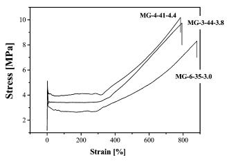
**Figure 10.** Influence of junction point functionality on stress—strain behavior of multigrafts with about 40% of PS content.
