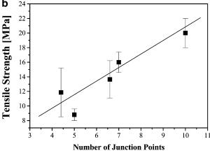
**Figure 6.** (a) Influence of number of branch points on (a) strain at break; (b) tensile strength of tetrafunctional multigraft copolymers with about 20% of PS.
