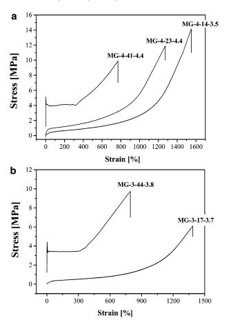
Figure 7. Influence of PS content on tensile properties of multigraft copolymers with about four junction points. (a) Tetrafunctional MG materials: MG-4-14-3.5 PS spheres; MG-4-23-4.4 PS cylinders; MG-4-41-4.4 lamellae. (b) Trifunctional MG materials: MG-3-17-3.7 PS spheres; MG-3-44-3.7 lamellae.
