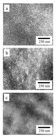
**Figure 2.** TEM images of hexafunctional multigraft copolymers with 21% of PS: (a) MG-6-21-5.3, (b) MG-6-21-3.6, and (c) MG-6-21-2.7.
