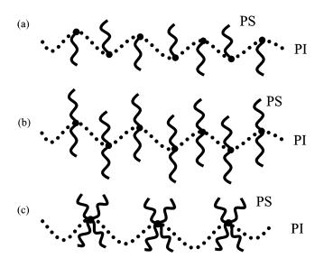
**Figure 1.** Illustration of multigraft copolymers based on PI backbone and PS branches with regularly spaced (a) trifunctional, (b) tetrafunctional, and (c) hexafunctional junction points.
