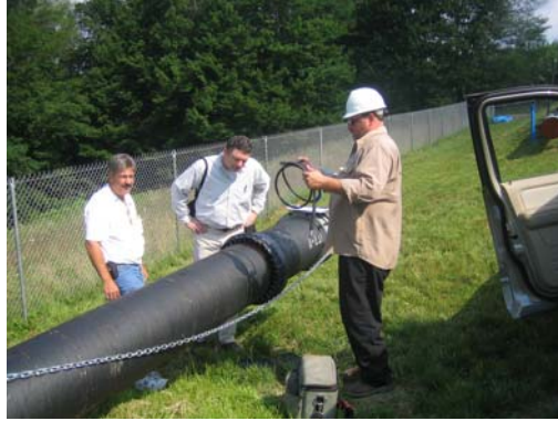
Figure 2 DOT and Industry Reps observe Application of transducer belt on 16" pipe
