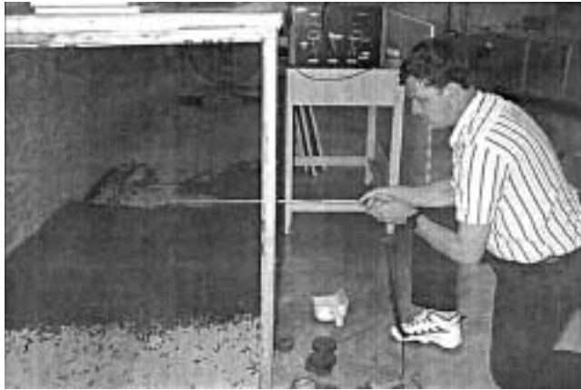
Figure 3—Measuring air velocity over a small tire chip mulch covering the hot plate.
