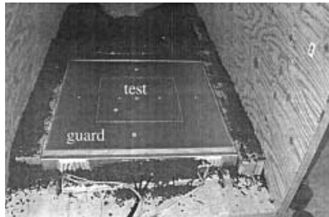
Figure 1—Guarded hot plate at the end of a wind tunnel.
