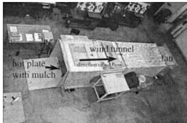
Figure 2—Top view of setup for forced convection heat transfer experiments.
