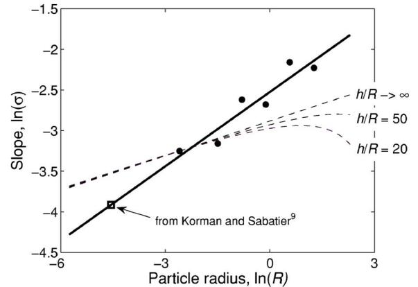
FIG. 3. Dependence of the slope of the resonance curves,  $\sigma$ , in region B on particle radius  $R$ . The experimental data from Table III are plotted as black circles. The power-law fit  $\sigma = \alpha R^\beta$  is given by the solid line ( $\alpha=0.08$ ,  $\beta=0.305$ ). This curve matches with data from Korman and Sabatier (Ref. 9). The dashed lines correspond to the analytical model for three values of  $h/R$ .
