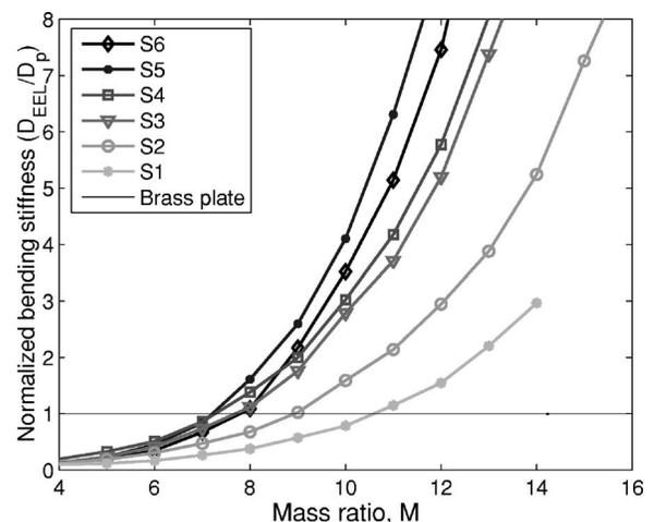
FIG. 8. Computed effective bending stiffness of the granular layer (see Table I) using the FEM-based inverse analysis for the equivalent elastic layer. Results are normalized by the bending stiffness of the metal plate.
