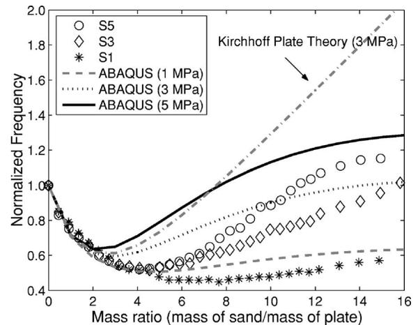
FIG. 6. Comparison of select experimental results with the two-layer plate model and the plate-EEL FEM model. The dash-dot line is obtained with the multilayer plate theory (Ref. 22) for  $E=3$  MPa while the FEM results are obtained for equivalent elastic layers with  $E=1, 3,$  and  $5$  MPa, respectively.
