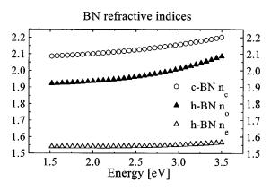
FIG. 4. BN refractive indices obtained from multiple-sample regression analysis fit and visible-light gVASE data ( $n_c$  c-BN: open circles,  $n_e$  h-BN: open up-triangles,  $n_o$  h-BN: solid up-triangles).
