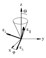
FIG. 2. Model of the geometry of the anisotropic h-BN thin-film microstructure from which the dielectric function model used in this work is obtained. The microscopic h-BN grain c axes are mapped onto the outer shell of a cone  $(0 \le \varphi \le 2\pi)$ . The cone axis is the sample normal. The thin-film optical anisotropy depends on the average c-axis grain orientation
