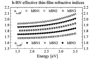
FIG. 1. Effective uniaxial thin-film refractive indices obtained from our h-BN samples and analysis of the visible-light gVASE data. Depending on the microstructure the thin-film optical anisotropy appears as uniaxially positive, isotropic, or uniaxially negative.
