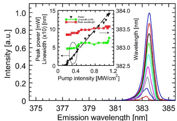
FIG. 4. (Color online) Emission spectra as a function of optical pump power measured at 0.15, 0.25, 0.35, 0.45, 0.6, 0.8, 0.9, 1.0, and 1.1  $\text{MW}/\text{cm}^2$  (from lowest to highest curve). The inset shows peak power (triangles, left y axis), emission wavelength (squares, right y axis), and linewidth (circles, left y axis, times ten) vs pump intensity curves.
