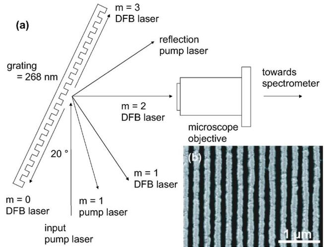
FIG. 3. (Color online) (a) Schematic representation of the optical pump experiment and relevant diffraction orders  $m$  of both  $\text{N}_2$  and ZnO DFB lasers. (b) Scanning electron microscopy image of the diffraction grating.
