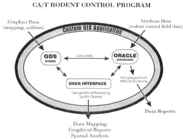
Figure 1. Functional diagram of the geographic information system designed for the CA/T rodent control program.
