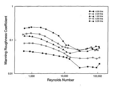
FIG. 2. Manning Roughness Coefficients as Function of Reynolds Number for Selected Rates of Wheat Residue
