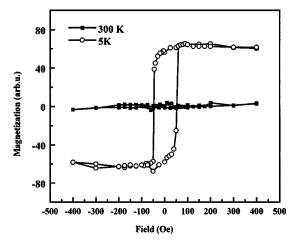
FIG. 3. Hysteresis loops for Co-C films before exposing the film to the interference laser at 5 and 300 K.
