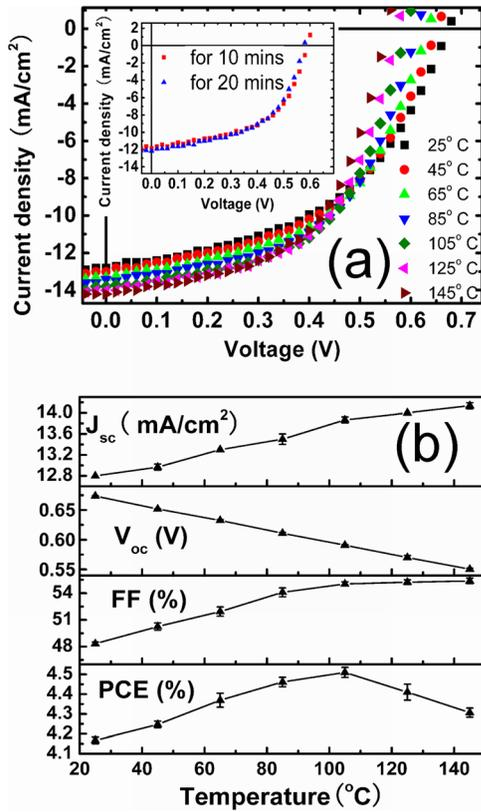
FIG. 1. (Color online) (a) Variation of  $J$ - $V$  curve with temperature. The inset shows the change of  $J$ - $V$  curve at 125 °C between after annealing 10 minutes and annealing 20 minutes; (b) Variation of photovoltaic parameters with temperature from RT to 145 °C.
