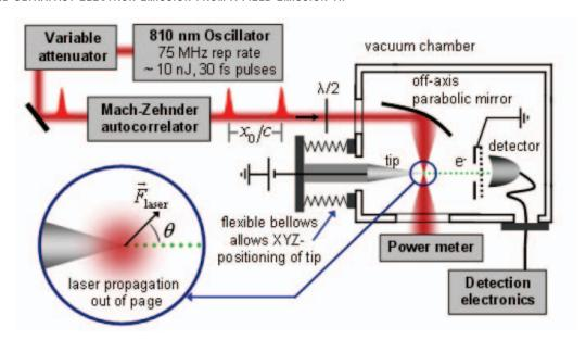
**Figure 2**. Experimental set-up. A femtosecond laser oscillator produces radiation pulses at a rate of 75 MHz. An autocorrelator provides time adjustable pump and probe pulses. The laser pulses are focused on a field emission tip to extract electron pulses. (For a more detailed description see text.)
