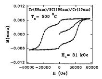
FIG. 4. Hysteresis loop for the 100-nm-thick SmCo film with a Cr underlayer of 20 nm annealed at 500  $^{\circ}\mathrm{C}.$
