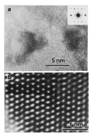
FIG. 2. (a) HRTEM image of Cr(80 nm)/PrCo(28 nm)/Cr(10 nm) film annealed at  $500 \,^{\circ}C$ . (b) HRTEM image of a crystallite in (a).
