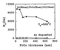
FIG. 1. Coercivity vs PrCo layer thickness for the as-deposited and annealed at 500 °C PrCo||Cr films with a Cr underlayer of 80 nm.
