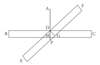
So if a slant is imposed on B, B will be at E and C will be at F. So the dividing line, at the exact vertical DM before, will be at DG during the slant. So the part of beam EF outside the vertical, marked GP, makes that side greater than half.
