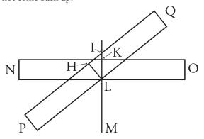
Let the beam lie on NO, and let the vertical be KLM. NO is divided equally. Put a weight on N. N will be at P, O will be at Q, KL will be at HL, so that IP will be greater than IQ by the amount HLI. Remove the weight and the low end will stay down, for the excess overlies on it like a weight.
