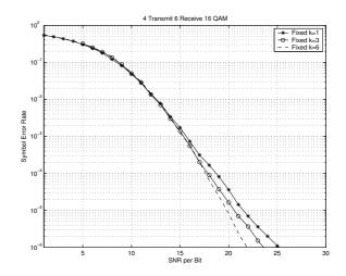
**Fig. 6**. 4 Transmit, 6 Receive 16-QAM SQRD with constellation size k=1, 3 and 6.
