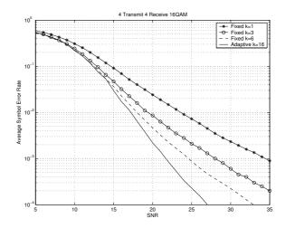
**Fig. 8**. 4 Transmit, 4 Receive 16 QAM, RSQRD with constellation size 1, 3, 6 and Adaptive with k=16.
