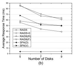
Figure 4. Comparisons of reconstruction times and average response times with respect to the number of disks driven by the Fin2 trace. The baseline reconstruction algorithm is PR.
