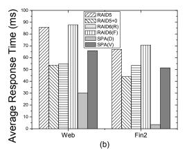
Figure 3. Comparisons of reconstruction times and average response times of the schemes based on the PR baseline algorithm.
