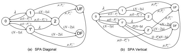
Figure 7. Reliability model of a RAID5 array with SPA protections. Figure 7(a) depicts the reliability model of SPA Diagonal, and Figure 7(b) depicts the reliability model of SPA Vertical.
