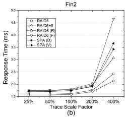
Figure 6. Comparisons of response time of various RAID systems for the traces: Fin1 and Fin2.
