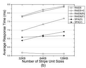
Figure 5. Comparisons of reconstruction times and average response times with respect to the numbers of stripe unit sizes driven by the Web trace. The baseline reconstruction algorithm is DOR.
