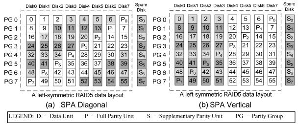
Figure 1. Two examples of SPA coverage and layout. Figure 1(a) depicts an SPA coverage with Diagonal Orientation, and Figure 1(b) depicts an SPA coverage with Vertical Orientation.
