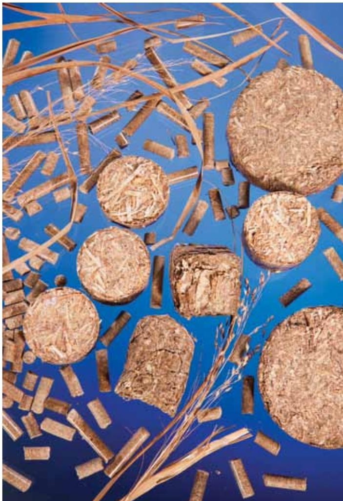
Switchgrass can be formed into pellets, cubes, and round briquettes that can be used to heat homes and businesses instead of fuel oil.
