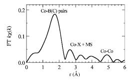
FIG. 2. A magnitude of the Fourier transform of  $k\chi(k)$  about the Co-based species in the PECVD grown boron carbide. The data are transformed for data taken from between 3.56 and 11.0 Å<sup>-1</sup>. The major peak is due to contribution of Co–B(C) atomic pairs. The peak at  $\sim$ 5 Å is associated with Co–Co pairs.
